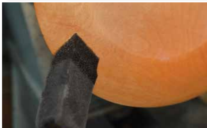
Step 5: applying size perpendicular to the rim
