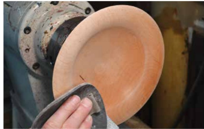
Step 3b: sanding with a backing pad
