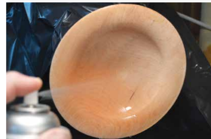
Step 2: spray shellac onto the surface
