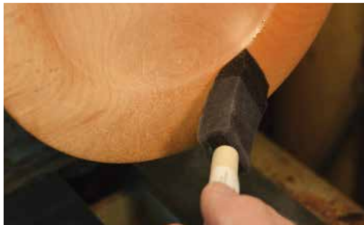
Step 4: applying the size parallel with the rim
