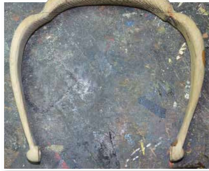
The handle, once cut out on the bandsaw and carved
