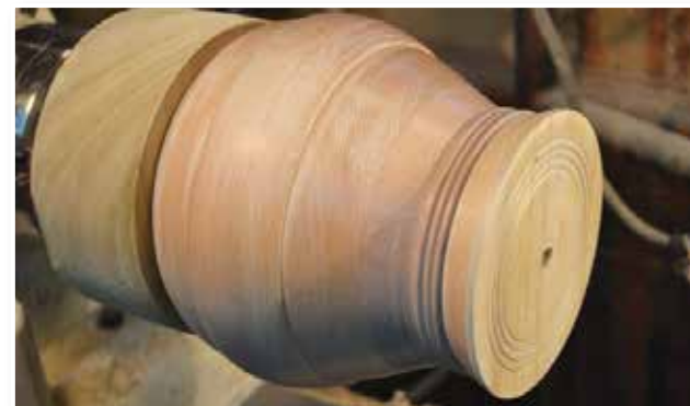
The piece placed on a fabricated jam chuck
