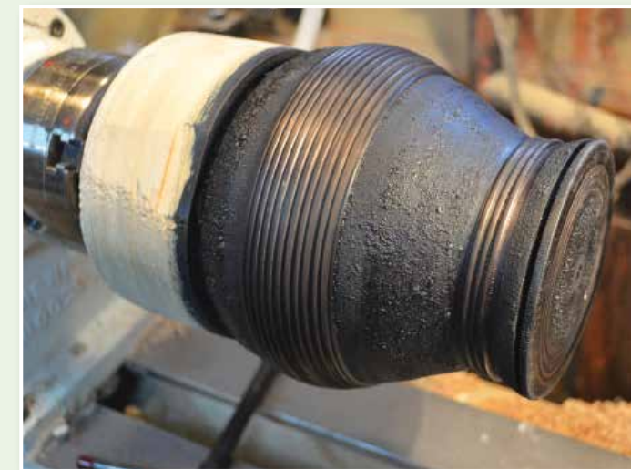
Building up layers of glaze mixed from spar varnish and black paint...
