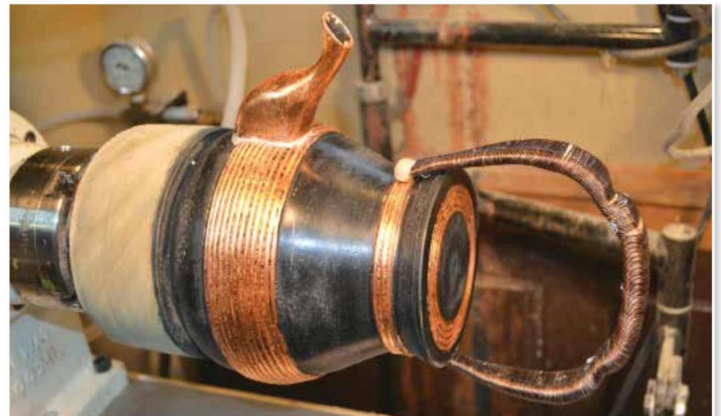
Applying copper leaf to the beading
