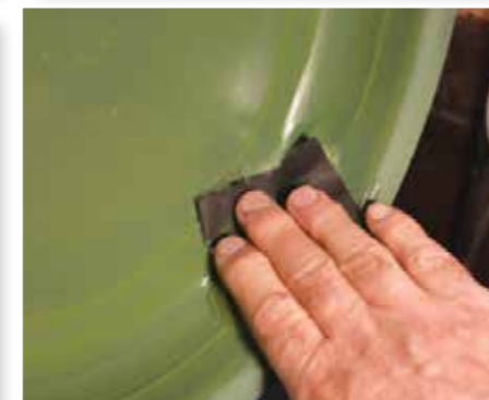
Step 6: the base coat is wet sanded...
