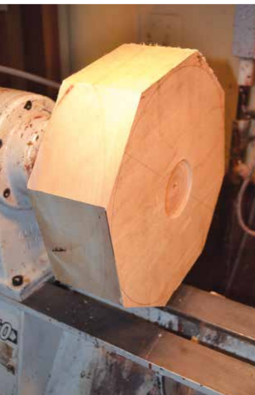
Step 1: creating a mortise for the expandable chuck
