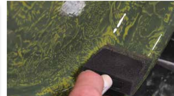
Step 18: applying a coat of varnish using a foam brush
