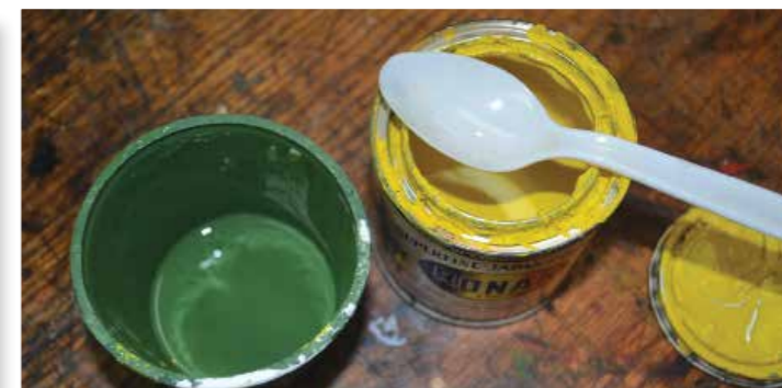
Step 3: the piece is then liberally coated with grain filler – or pore filler
