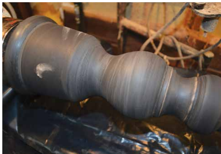
Step 3: the base coat sanded and ready for clay and copper leaf application
